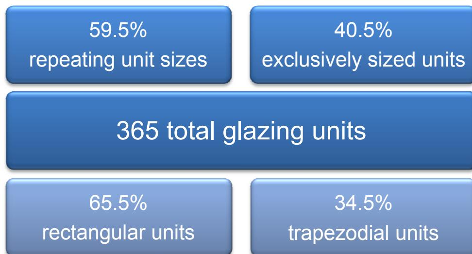
**Figure 21:** Break Down of the Curtain Wall Glazing Units
